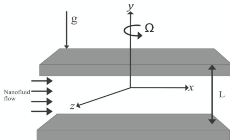
*Figure 1: Configuration of a two-phase Nanofluid flow*
