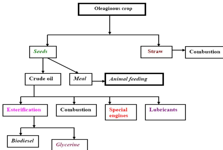
Figure9. Flow chart of biodiesel production (Omer, 2006).
