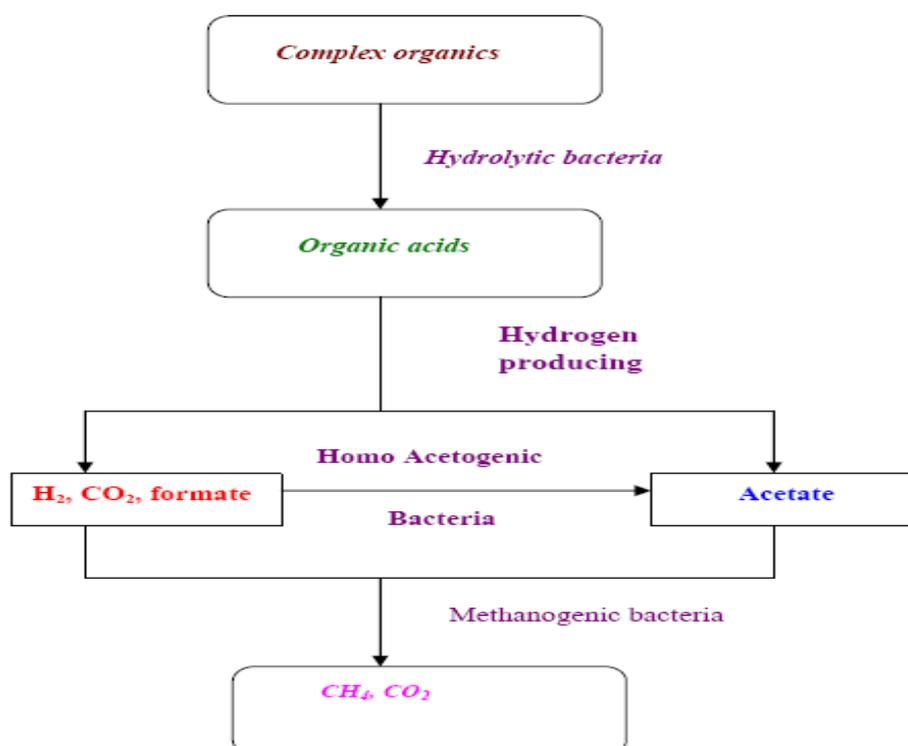
**Figure3.** Biogas production process (Omer, 2003).
