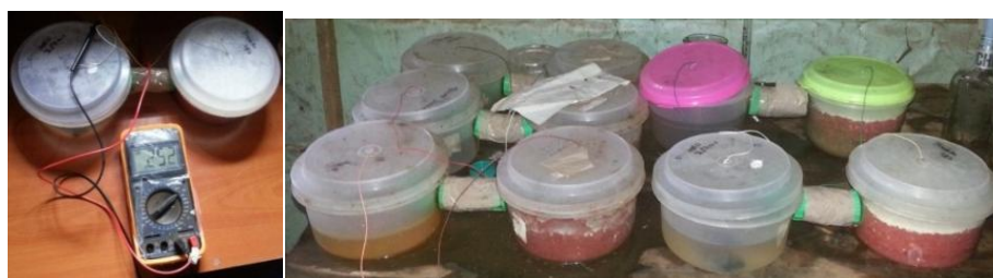
Figure2.1. Double chamber MFC with a voltmeter and batch MFC.
