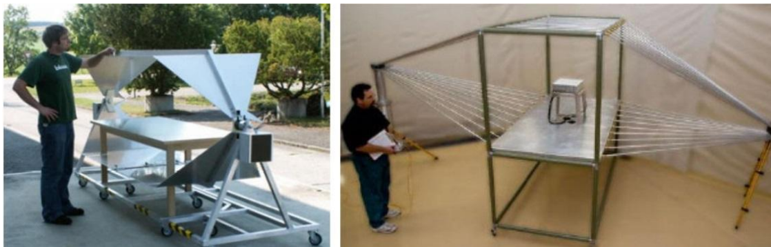
Fig1. Compact test-beds for testing electronic apparatus sustainability to HEMP. a- Montena Technology, б - Applied Physical Electronics
