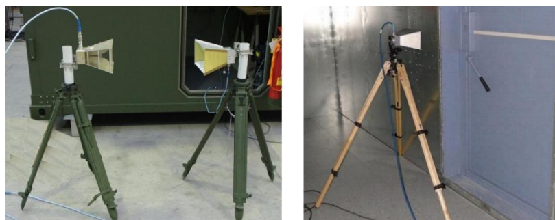
Fig7. Adjustment (resetting to zero) and usage of device for evaluation of shielding effectiveness
