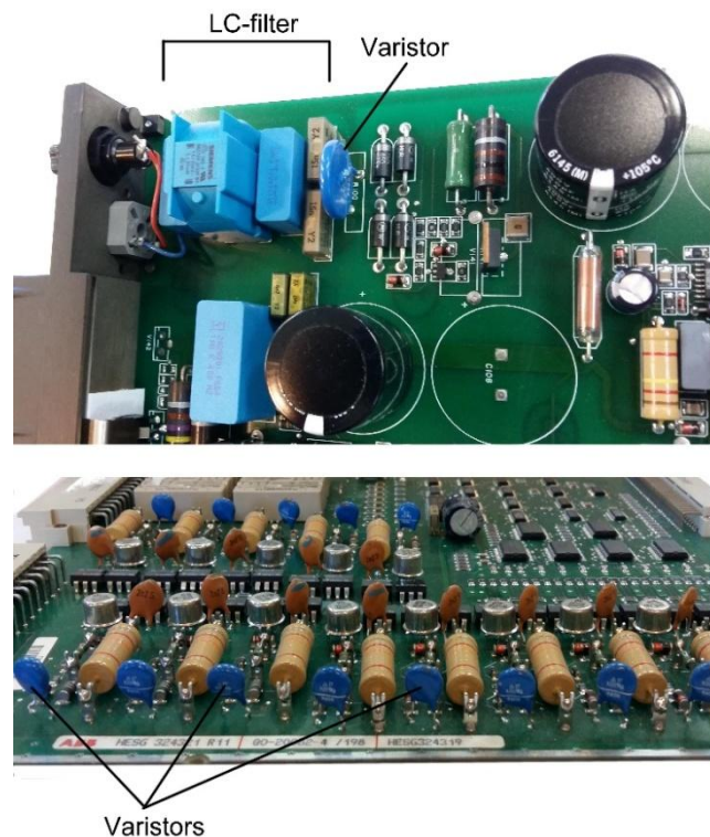
Fig10. Usage varistors in power supply (up) and logic inputs (down) of relay protection
