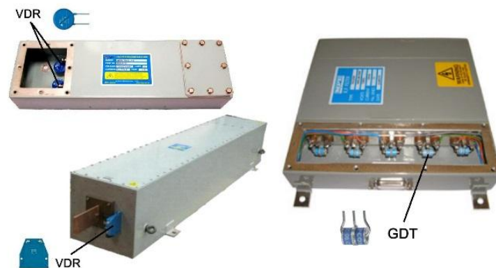
Fig6. Some HEMP filters equipped with HV pulse protecting elements. VDR – varistor, GDT – gas-discharge tube.
