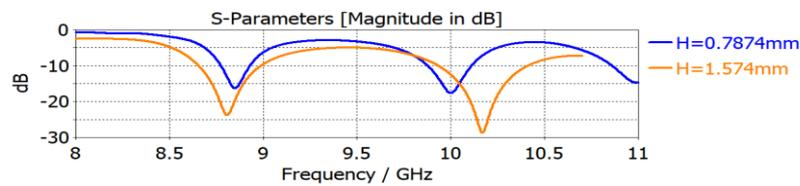
Fig6. Frequency response  $S_{11}$  for a substrate with two thicknesses of 0.7874mm and 1.575mm
