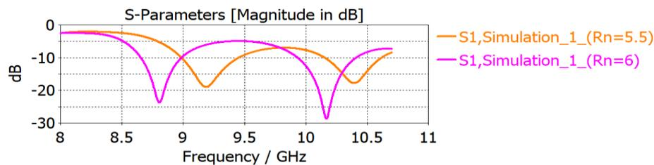
**Fig4.** For every 0.5 mm change in the circle diameter, the frequency response is shifted about 400MHz.
