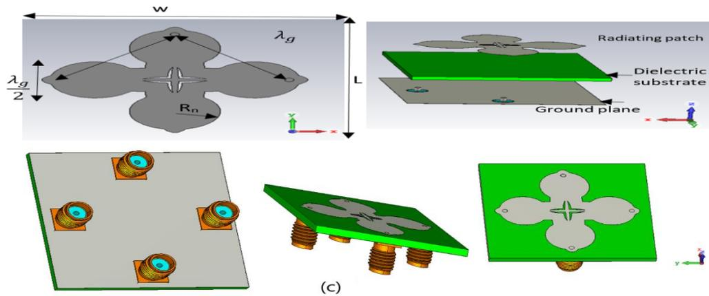
**Fig1.** Antenna configuration, (a) radiating patch. (b) Three layers of expanded antenna structure, (c) 4 port configure.
