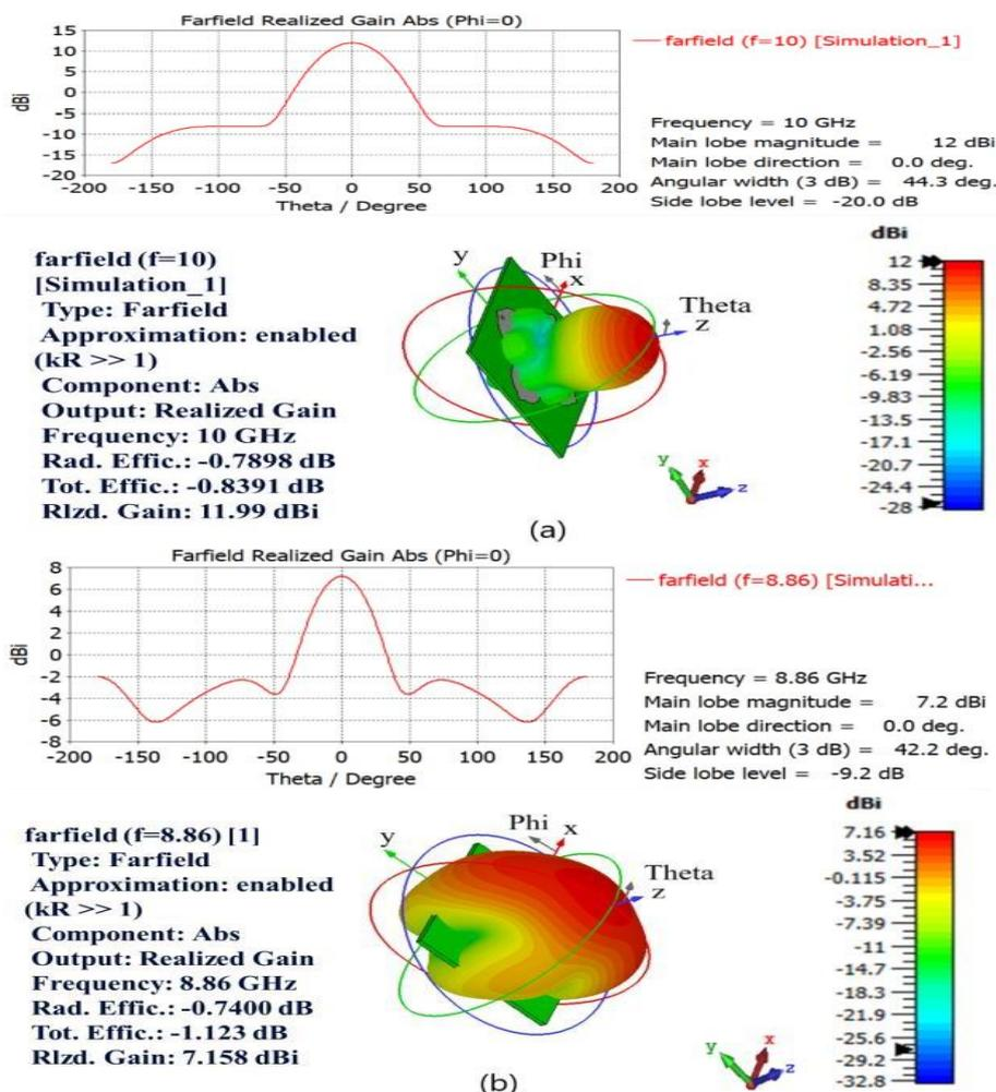
Fig8. The antenna radiation pattern for two frequency bands (a)8.9 GHz and (b)10 GHz in Cartesian and 3D coordinate.
