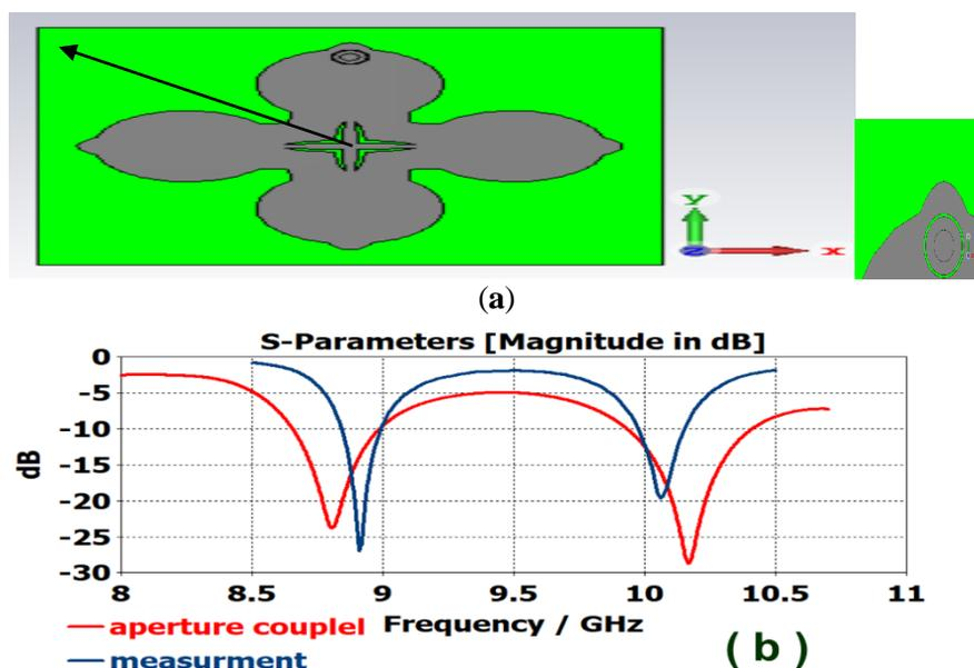
Fig12. Antenna shape with aperture coupler feeding (a), and S11 parameter response compared to without aperture coupler (b).
