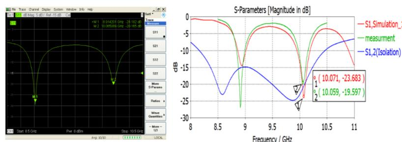
**Fig10.** Return loss and isolation for two ports, frequency response for two bands, and measurement result.
