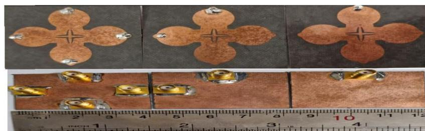
**Fig9.** Built-in antenna structure with one, two, and four ports
