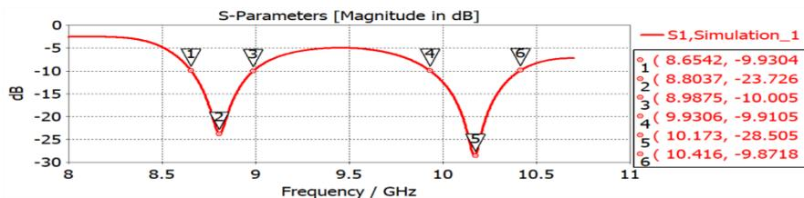
Fig7. Diagram  $S_{11}$ , the frequency response for two frequency bands
