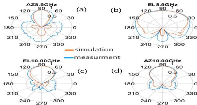
Fig11. The measured pattern compared to the simulated results
