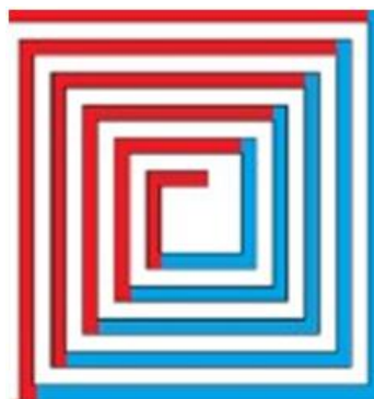
Figure3. Represents the previous example with a negative displacement in red and the positive displacements in blue. Eventually implementing these changes into the code provided by NASA was harder than it seemed and the square spiral path was dropped
