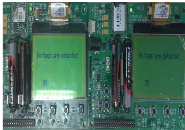
Fig3. LCD panels of two Readers displaying “No tag detected” message. (Readers are ON, Tag is OFF)
