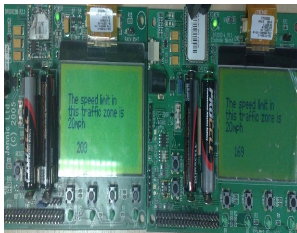
Fig4. LCD panels of two Readers displaying speed limit information.
