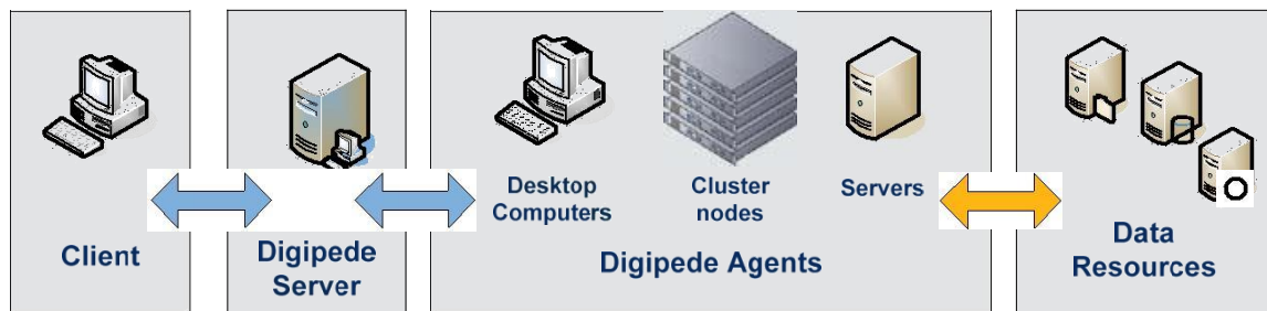
Figure: Digipede Network Topology
