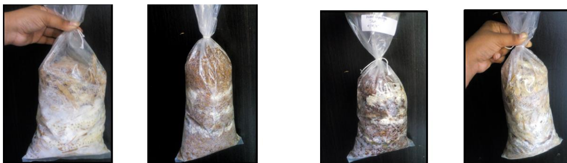
Fig3. Packing of 50% vegetable waste+ 50% agro waste (a)paddy straw (b)rice husk (c)wood shavings and (d)sugarcane bagasse
