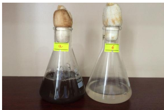
Figure1. Color change of reaction mixture during formation of silver nanoparticles by Actinomyces spp.NSX-333 : a-experiment, b-control
