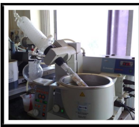
Fig6. Rotor evaporator used for concentration of solvent
