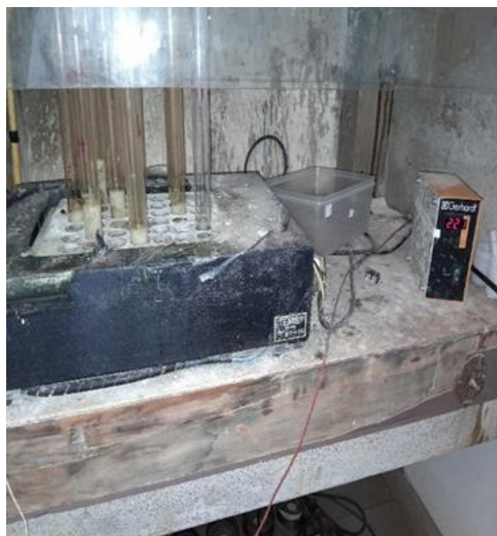
Figure3. Digestion of the milk samples in a block digester.
