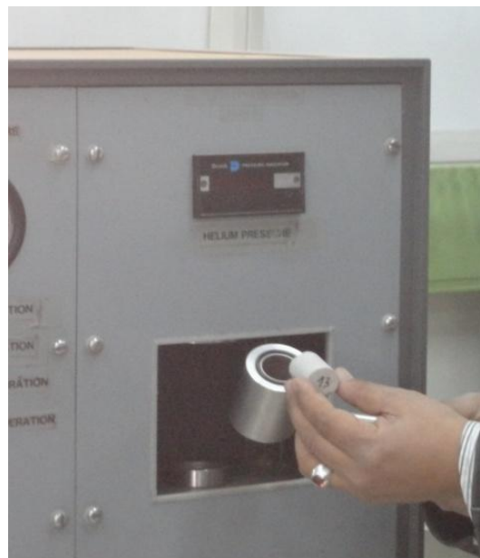
Figure9. Total porosity analysis of rock plug using helium porosity (AGOCO-Lab)
