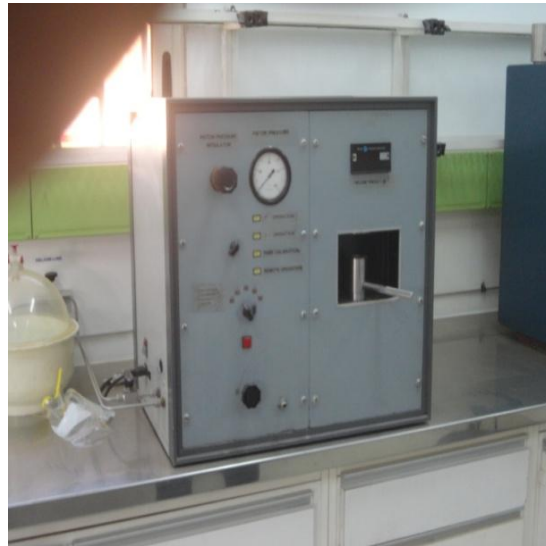
Figure7. Corex Helium Porosimeter at AGOCO Lab
