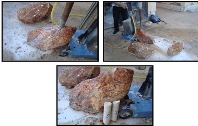
Figure6. Rotary core cutting machine at AGOCO Lab
