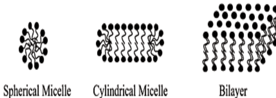
Fig3. Schematic illustration of the three most commonly observed geometrical shapes of surfactant micelles [11]
