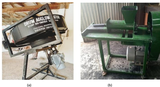
Figure4. Briquetting Technologies (a) Drum Agglomerator (b) Screw Press
