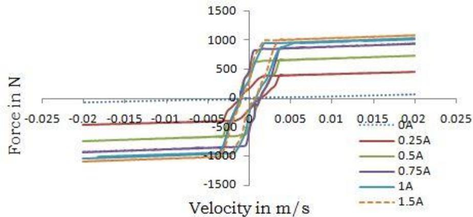
Figure 7. Force Vs velocity for MR Damper prototype
