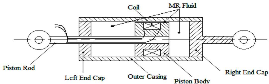
Figure 1. Monotube MR damper
