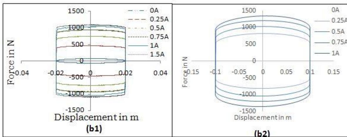
Figure 15. (b): Comparison of experimental data (b1) with simulated data (b2) for Force Vs displacement
