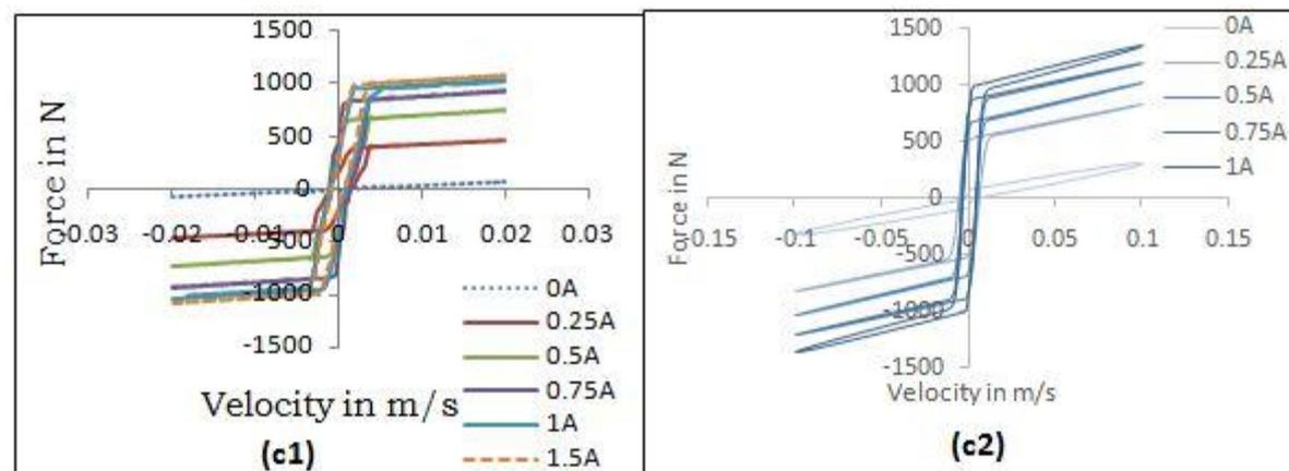
Figure 15. (c): Comparison of experimental data (c1) with simulated data (c2) for Force Vs velocity
