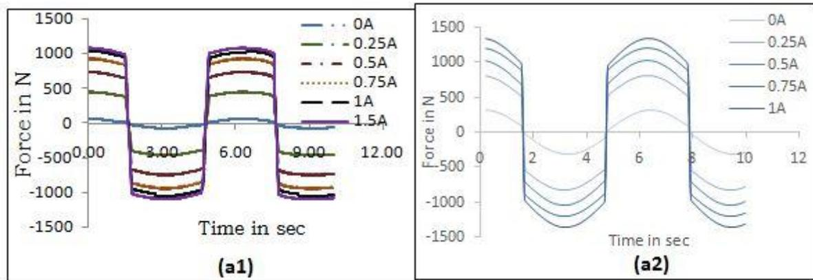
Figure 15. (a): Comparison of experimental data (a1) with simulated data (a2) for Force Vs time
