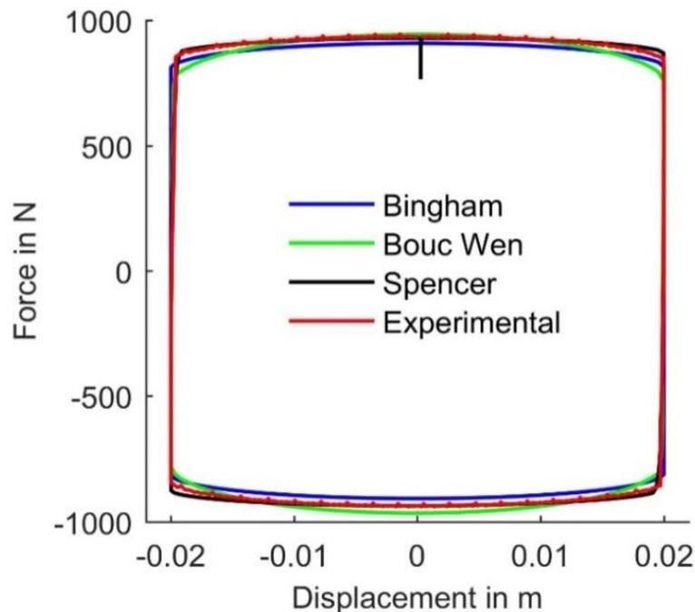
Figure 12. Output force Vs displacement of damper prototype
