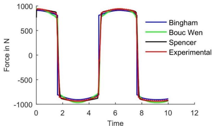
Figure 11. Output force Vs time of damper prototype
