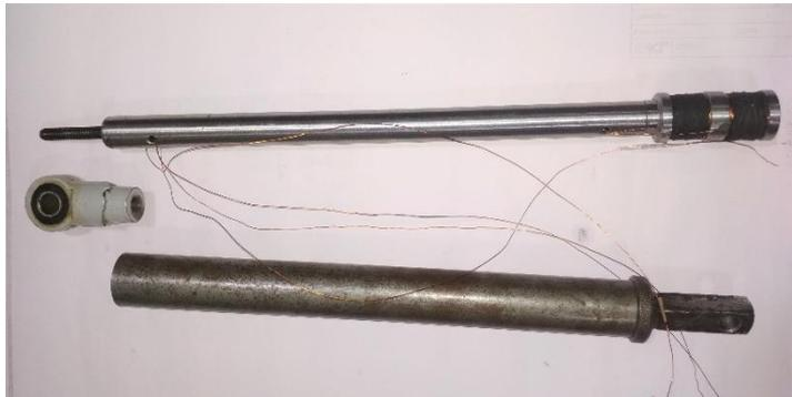
**Figure 2.** Piston rod with solenoid and cylindrical casing
