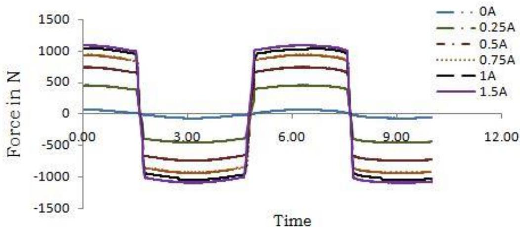
Figure 5. Force Vs Time plot for MR Damper prototype
