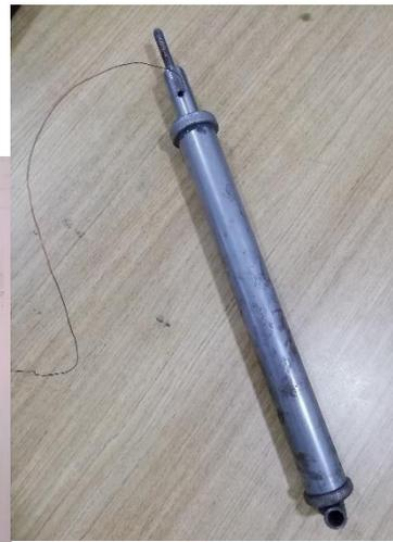
**Figure 3.** Assembly of the damper
