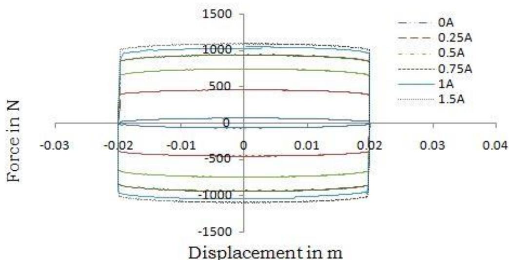
Figure 6. Force Vs displacement for MR Damper prototype
