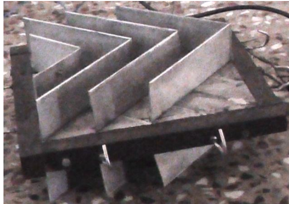
Figure2. Plate with V-Fins
