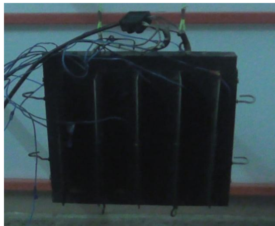
Figure3. Plain Blackened Vertical Plate with Fins
