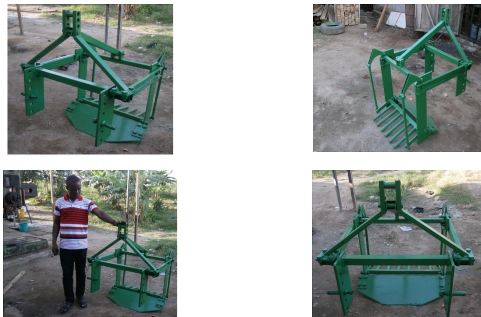
Figure7. The fabricated mechanical yam harvester.
