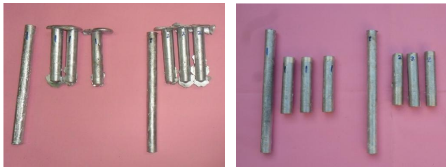
Fig7. Casting of samples and after machined samples
