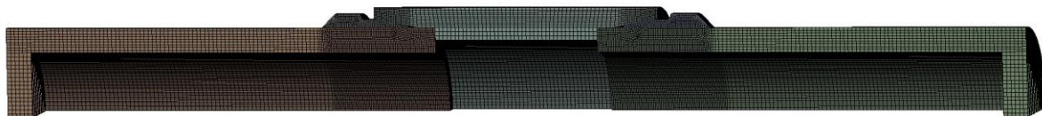
Figure3. Grid setup of pipe joints
