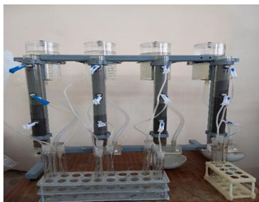
Fig1. Laboratory setup for ascending fluid flow.
