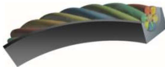
Fig6. Model of connecting bent rope and frictional lining in three dimensions.
