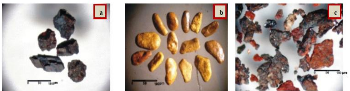
Fig31. Stereophotograph of (a) ilmenite, (b) leucoxene and (c) hematite, W. Abu Rusheid stream sediments, SED, Egypt
