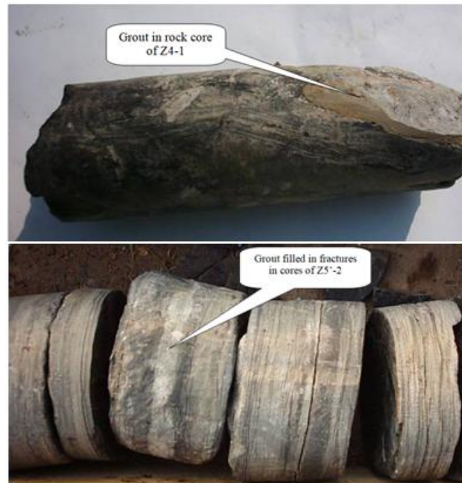
Fig7. Core samples at select grout holes
