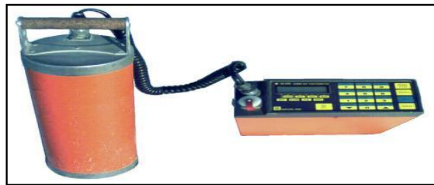
Fig.11 Multi-channel GS-256 portable spectrometer with gamma ( \gamma ) sensor (9903). Geophysica, LTD Czechoslovakia.
