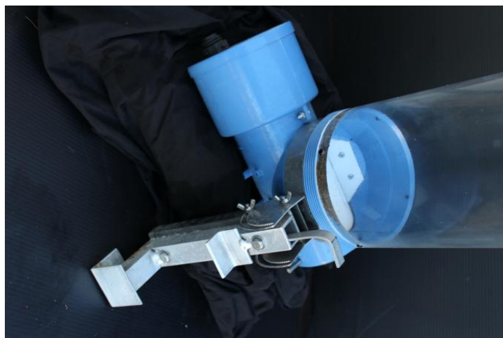
Figure 5. Image of the back view of an automatic feeder mount for a 1.8-m diameter circular rearing tank.
