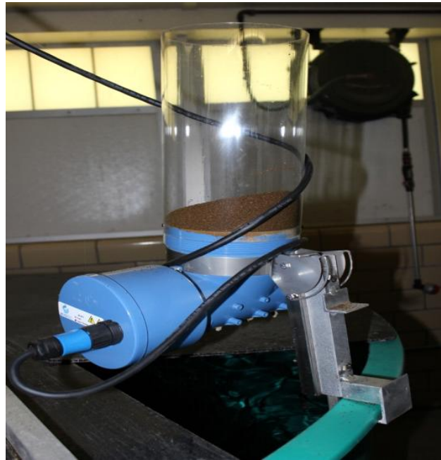
Figure 1. Image of an automatic feeder mount for a 1.8-m diameter circular rearing tank in use during hatchery operations.
