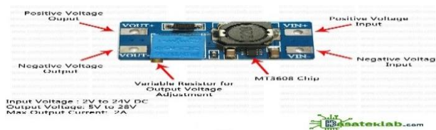
Fig3.2: MT3608 DC To DC Step Up Boost Converter Module
