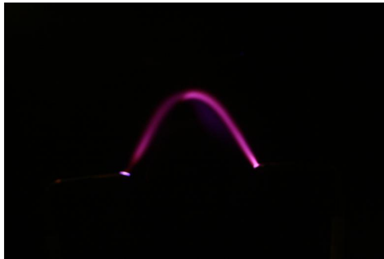
Figure9. Arched form of glow discharge
