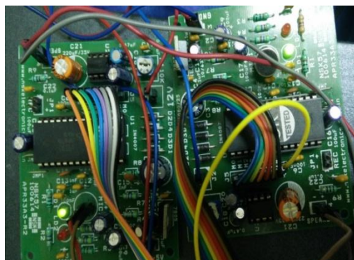
Fig5.4. Audio playback board used for vocal message
