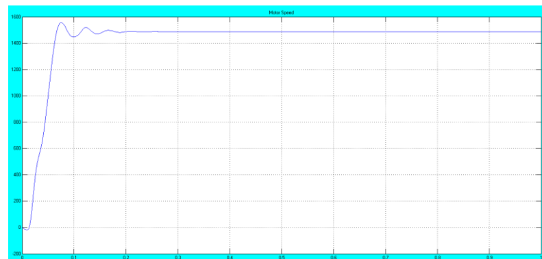
Fig20. Simulation result for asynchronous motor speed
