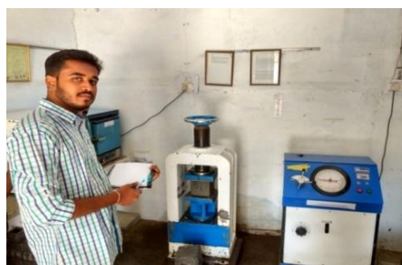
Figure2. Setup of Compression compressive strength testing machine
