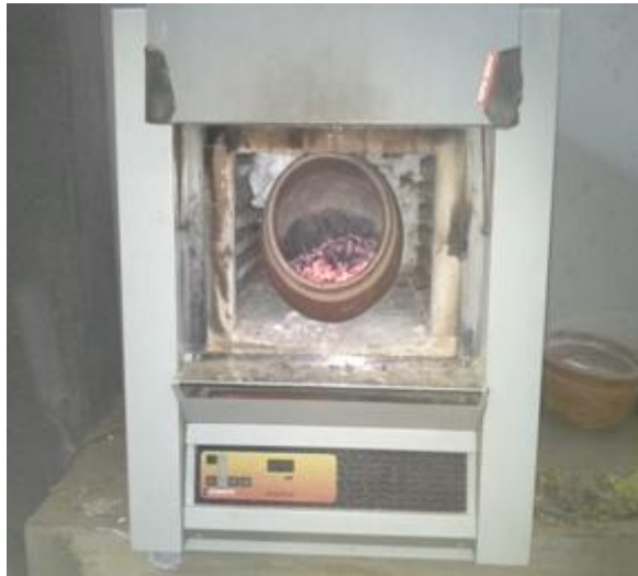
Plate3. Converting Cassava Peel to CPA (placed in earthen pot)
