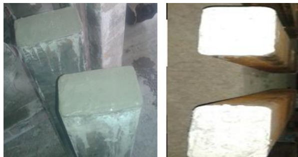
Fig. CFST columns before and after application of curing compound
