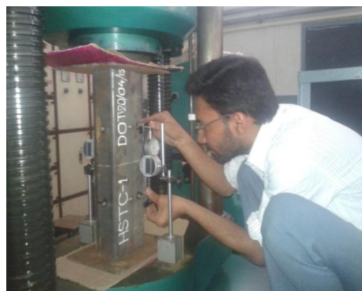
Fig. Test set up of CFST Column for axial loading
