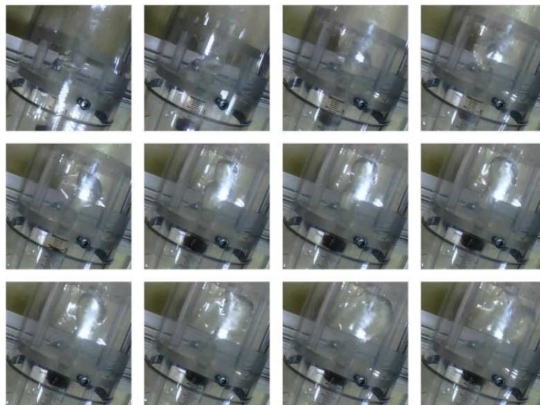
Figure8. Frame-by-Frame display of Team 1’s Column 17 showing the whirlpool effect (time evolution from left to right row-wise)
