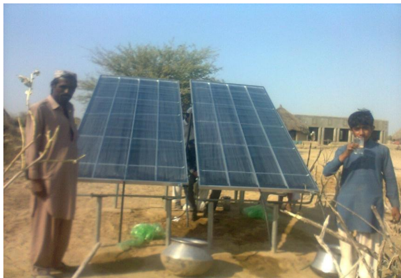
Two unit of solar desalination at Goth Nawab Ji Dhani, Umerkot, Sindh
