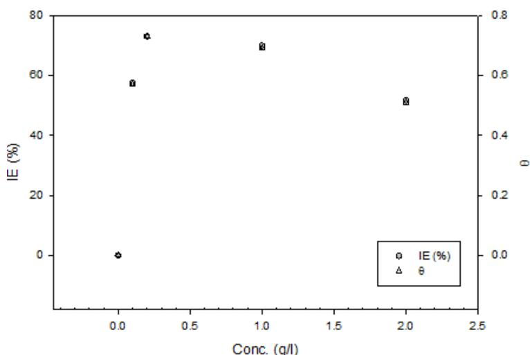
**Fig3.** Graphical representation of IE and  $\Theta$  as a function of NPK concentration in the solution
