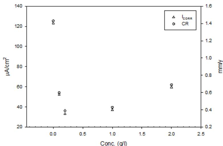
**Fig2.** Graphical representation of  $I_{CORR}$  and CR as a function of NPK concentration in the solution
