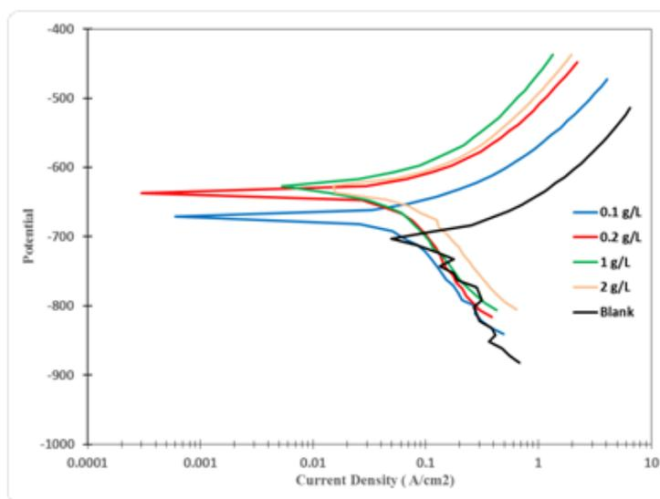
**Fig1.** Potentiodynamic curves for mild steel in water of the tank number 2204 in the presence and absence of various concentrations of inhibitors.
