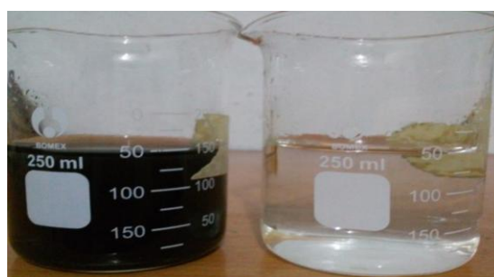
Fig8. Solution with the combination of CH 3 COOH and pine oil before (left) and after (right) flotation
