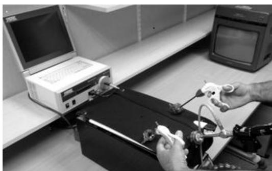
Figure2. Self constructed laparoscopy training box with Tele Pack®, Endopath® ports, Hopkin 2® 0-degree laparoscope, Ethicon® instruments, calibrated (Scale) and non-calibrated (Control) for working ports.
